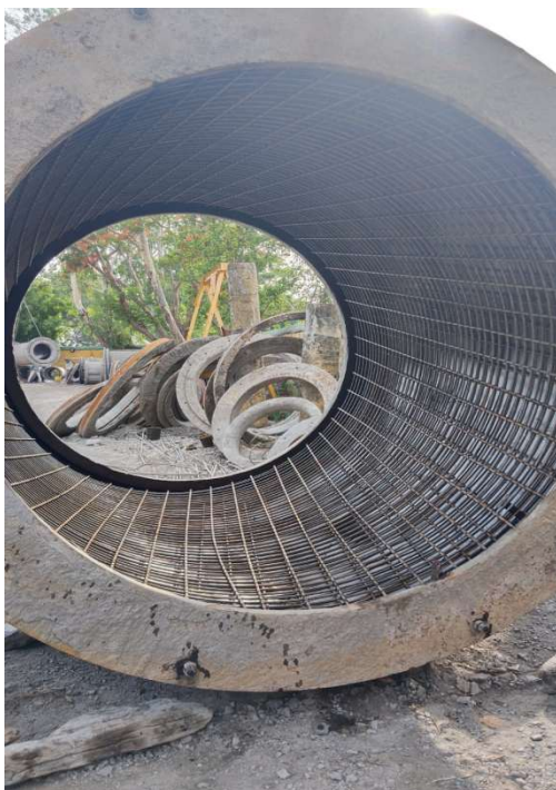
Fig (i): 2000mm dia NP4 Grade Jack Pushing Type RCC Hume Pipes fitted with MS Collar
