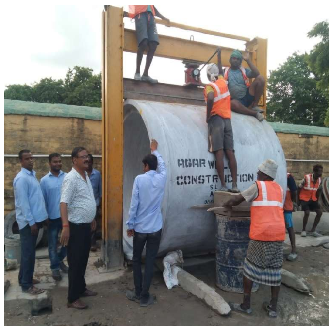
Fig (v): Three Edge Load Bearing Test being performed on 2000mm dia NP4 Jack Pushing Pipes
